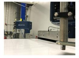
The IR-3000 will provide non-contact, instant, continuous measurements in real time, capturing thousands of measurements per second. It is insensitive to material variations like particle size or color. The production environment is removed from the measurement calculations by the software so things like small gaps, inert material, foreign objects, or conveyor belts and screws can be programmed to not interfere with the measurements being taken.
