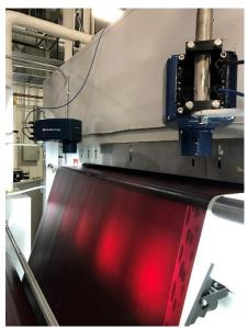
There are many locations throughout manufacturing that our sensor can be used. These locations are often determined by the space availability and accessibility on the machinery as well as manufacturer's control plan. After installation of the IR-3000, a manufacturer can continuously monitor the process and control the thickness and moisture content either manually or automatically from readings of the IR-3000 online sensor
